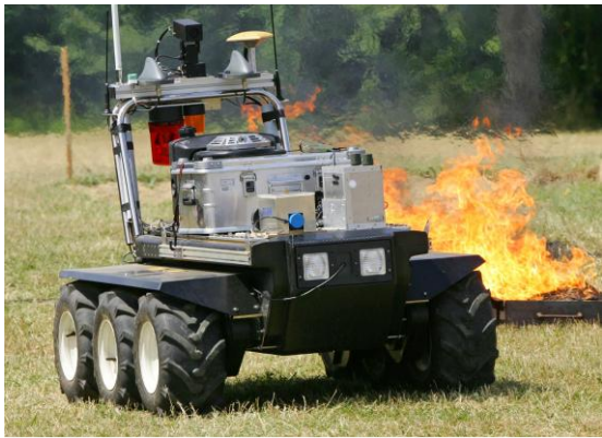
Figure 3: The experimental CBRNE platform Kutusow. The metal boxes contain various CBRNE sensors which may trigger an alarm both locally and at the control station 11
