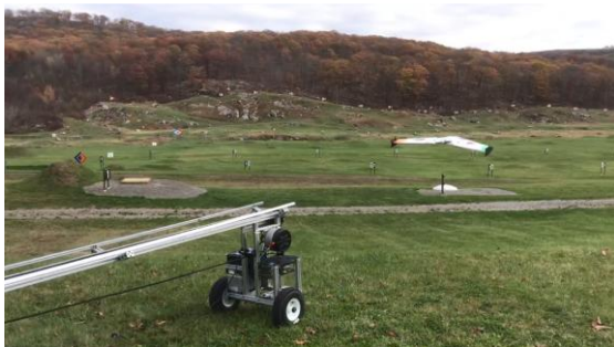
Figure 5: Field testing of the DARPA launcher and a ZephyrII fixed-wing sUAS at Range 11, West Point, NY 15
